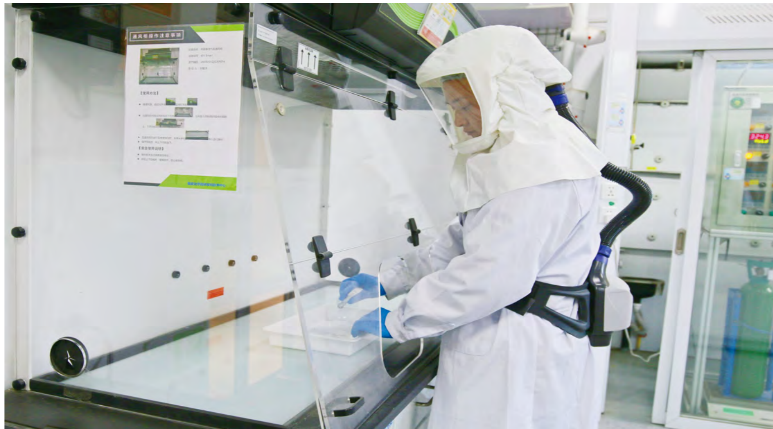
△ Zhejiang Research Institute of Chemical Industry provides employees with electric air supply protective respirators to prevent inhalation of harmful gases and ensure experimental safety
